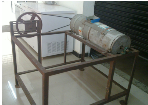
Fig.1. Peeling machine developed by CEPCI
