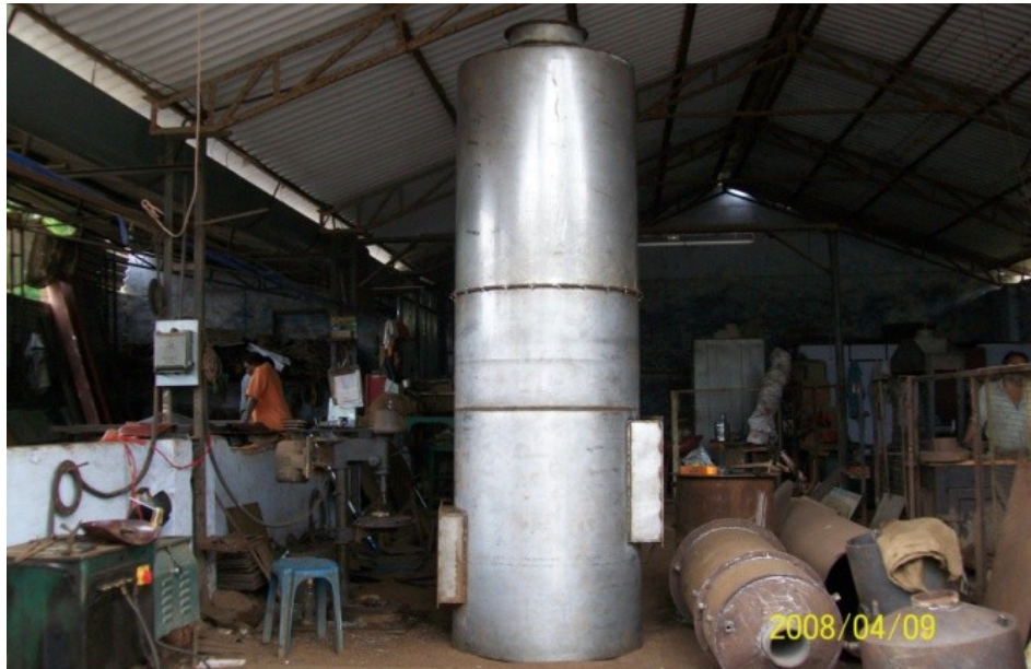
Fig3: The scrubber ready for installation at roasting unit
